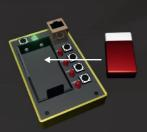
2. Connect clip to the firework safety fuse, as close to the end as possible.
